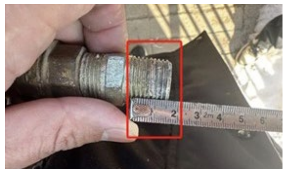
Hebei Natural Gas measured the effective length of the screw nipple
